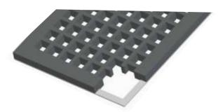
**RUBBER SCREENS WITH STEEL FRAME**, made of angle bar and steel rods – can also pose as a self – supporting deck, used mainly for prescreening in tough conditions. They are mounted using side rubber rods.
